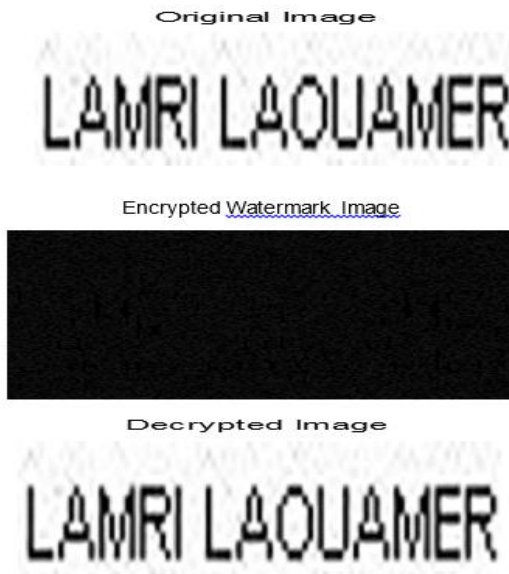
Fig. 14. Illustration of RSA-based Encryption and Decryption on the Watermarked-Signal
